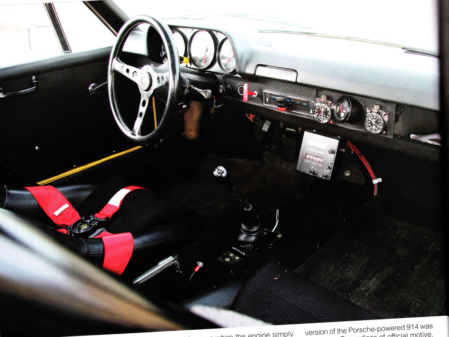
914-6 GT interiors vary; this one has GT door panels and gauges (note fuel gauge in radio position) but retains lower dash trim and carpeting. Rally equipment was added. Front trunk takes a spare tire between the bigger fuel tank and the oil-cooler ducting.
